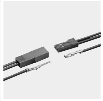
The RCY connector is a compact, 2.5mm (.098") pitch wire-to-wire connector for use with a variety of circuits, from signal circuits to power supply circuits, in electrical equipment which is becoming more and more compact. The employment of a free spring contact method ensures stable contact performance, and superb working efficiency of insertion and removal.
